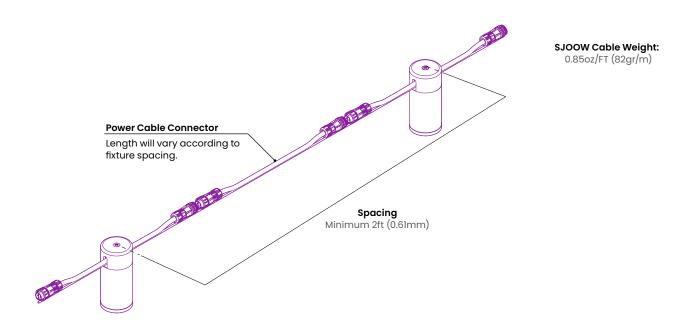
The length of "B" Power + Connector varies depending on the spacing between the lights.
