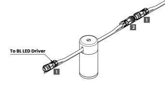
\*The length of **B** (Power Cable Connector) varies depending on the spacing between the lights.
