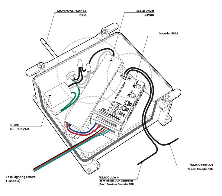
\* All devices in a DMX512 system must be connected in a "daisy chain" fashion.
