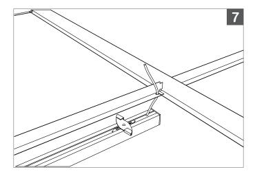
While gradually pulling the wire through, gently raise the luminaire up until it makes contact with the T-bar.
