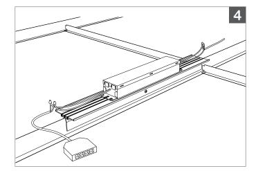
Connect the One to Four Wire Quick Connect to the 24VDC output of the LED Driver.
