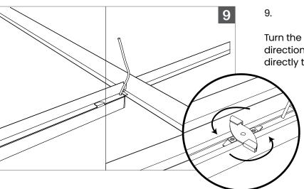
Turn the Rotary Mounting Clip in a clockwise direction, and securely fasten the Luminaire directly to the T-bar.
