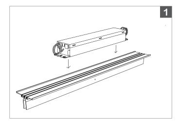
Secure the LED Driver to the Mounting Rail. Remove adjacent ceiling tiles and install Mounting Rail over top of T-bar.
