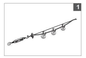
1. When assembling the Suspension Kit, fasten the **Spotglobe** wire into the assembly with Clamps.
