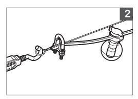
2. The Aircraft Cable should have a minimum 1/8th (3mm) diamater to handle weight of **Spotglobe** up to 100'.
