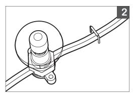
2. Use Insulated Wire Clips when installing **Spotglobe**. For a secure harness, please use a minimum of two clips per foot.
