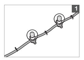
1. Ensure that **Spotglobe** wire is taut and controlled to mounting surface before permanently mounting.
