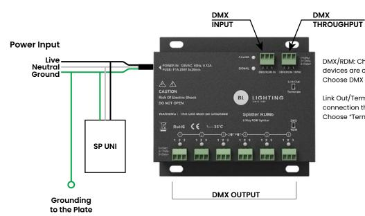
DMX/RDM: Choose the RDM setting if RDM-enabled devices are connected to the DMX outputs. Choose DMX otherwise.
