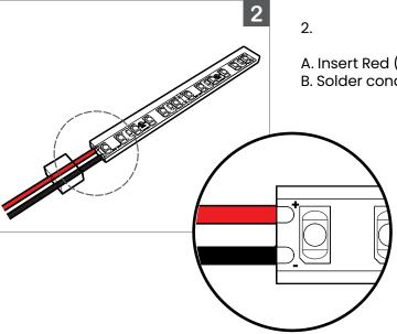
A. Insert Red (+) and Black (-) conductors through End Cap. B. Solder conductors directly onto PCB at assigned location.
