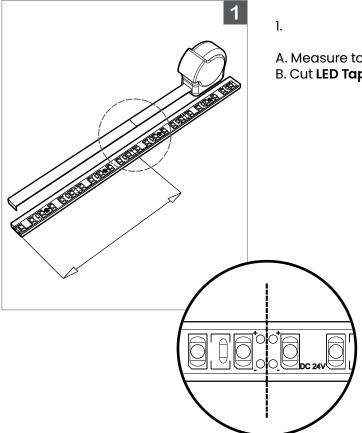
A. Measure to required length of **LED Tape**. B. Cut **LED Tape**.
