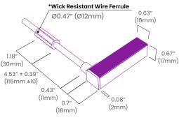
\*The Wick Resistant Wire Ferrule is built into the lead wire, 4.5" (115mm) from the BL Neonview Termination Connection, for additional moisture ingress protection. Removal of the Wick Resistant Wire Ferrule may void your warranty.
