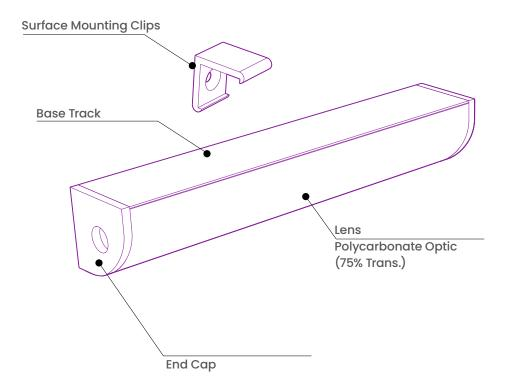
Each 6ft length of LED Profile is shipped complete with End Caps and Mounting Clips.
