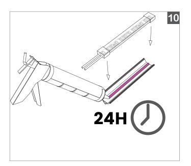
**IMPORTANT:** Allow adequate time for adhesive to cure, a minimum 24 hours is recommended. Refer to the instruction on the specific adhesive being used for guidance.
