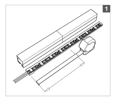
Measure **BL Fixform** in parallel with **BL Flexform** for accurate coupling of components prior to cutting.
