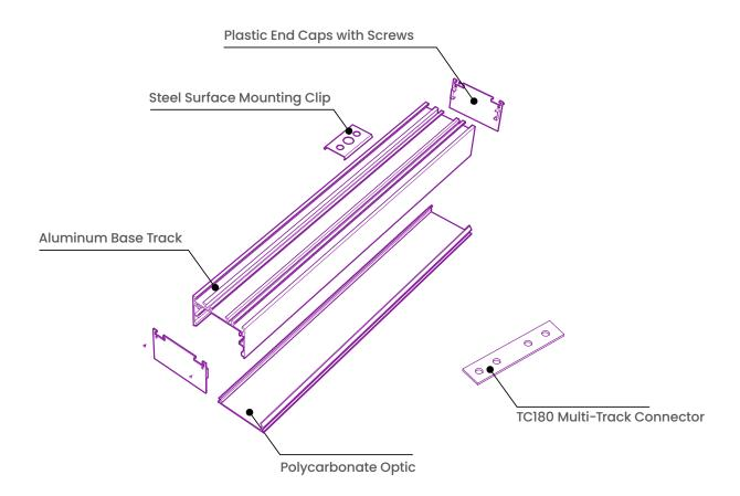
**S4930** is designed to house two side by side lengths of **BL Flexform LED Tape**.
