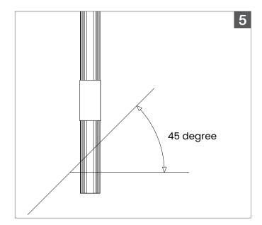
Measure desired length and start the cut from the top **Base Track** piece.
