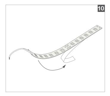
Remove the double-sided tape backing from the LED, if applicable, and secure the **BL Flexform LED Tape** into the Base Track using the adhesive provided on the LED, and/or adhesive tube.
