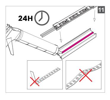
Secure **BL Flexform LED Tape** gently along the length, without bending or pulling up. Bonds should be held in place until adhesive has fixtured. Masking tape may be used along the length of the LED for this purpose.
