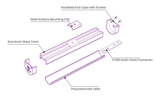
Each 6ft length of LED Profile is shipped complete with End Caps, Mounting Clips and TC180 Multi-Track Connectors with hardware.
