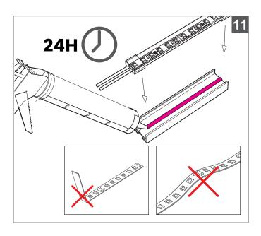
**IMPORTANT:** Allow adequate time for adhesive to cure, a minimum 24 hours is recommended. Refer to the instruction on the specific adhesive being used for guidance.
