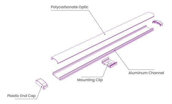
Each 6ft length of **\$1905** is shipped complete with End Caps and Mounting Clips.
