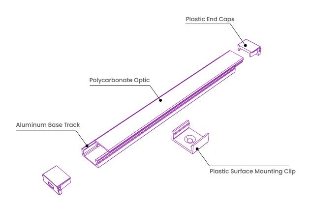
Each 8ft length of LED Profile is shipped complete with End Caps and Mounting Clips.
