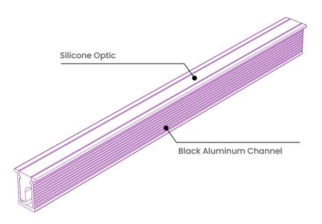
RN1007 is designed to be flush recessed into a wooden surface.
