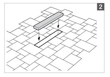
2.Insert foam base. Add or shave down foam base until optimal height is acheived for flush installation of **RC21**.
