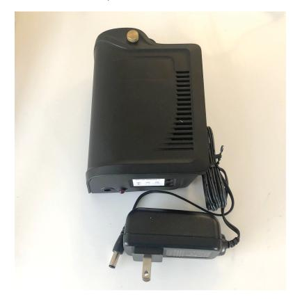
Connect the jack plug into the socket in the back, and the **Orion** is now ready for connection.
