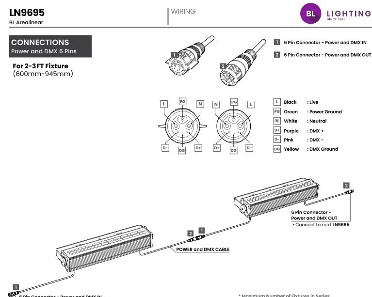
6 Pin Connector - Power and DMX IN Connect to Power Supply (100 - 277VAC)
