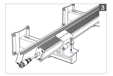
Attach the fixture to the mounting arm by using the through-mounting holes on the brackets with suitable fasteners.
