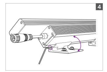
Tilt LN6260 at desired angle. Re-Tighten with Hex Key
