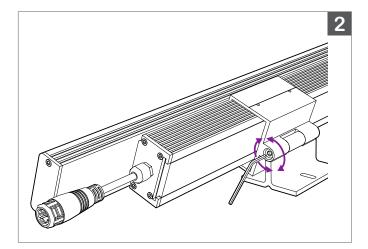
Loosen the mounting bracket with Hex Key, and tilt the fixture to one side to reveal the mounting brackets.
