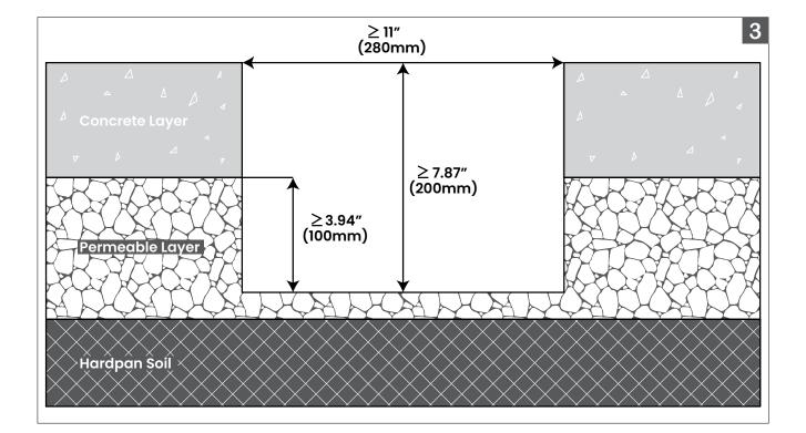
Depth of cutout in ground surface will depend upon the depth of permeable layer, concrete top layer, and concrete footing size required.
