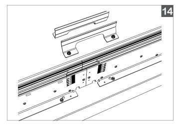
Secure Channel in place, and maintain secure connection and alignment with subsequent channel lengths using the Channel Connector Brackets.
