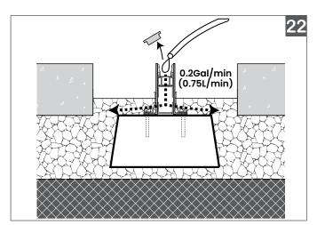
Fill the hole surrounding the Channel and cable conduits with the permeable fill (drainage gravel, pea gravel, or sand).
