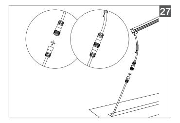
Verify wiring to the LED Driver, remove protective end cap, and connect to power using Quick Connects and test.
