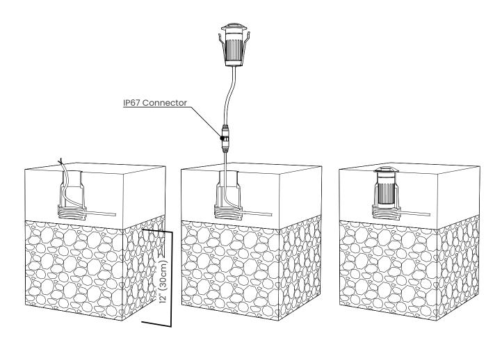
Prepare the ground, providing proper support for the mounting boot and install an adequate drainage system according to the application. Pipes may be installed in soft or hard ground to provide adequate drainage. For soft ground installations, drainage material such as pea gravel must be installed to a minimum depth of 12" (30cm). Minimum drainage rate 0.2Gal/min (0.75L/min) Luminaire should be installed only once adequate drainage is confirmed and mounting boot is dry and clean of debris.
