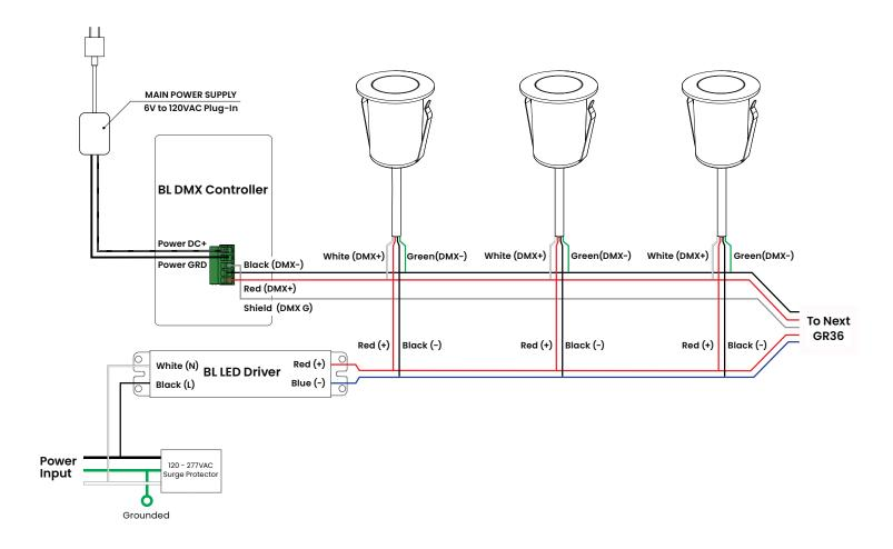
Solid State Lighting is sensitive to power fluctuations. Surge protection is highly recommended for all LED lighting products and should be on a dedicated circuit to protect against premature failure. Lack of surge protection may void your warranty.
