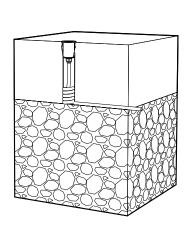
Prepare the ground, providing proper support for the mounting sleeve and install an adequate drainage system according to the application. Pipes may be installed in soft or hard ground to provide adequate drainage. For soft ground installations, drainage material such as pea gravel must be installed to a minimum depth of 12" (30cm). Minimum drainage rate 0.2Gal/min (0.75L/min) Luminaire should be installed only once adequate drainage is confirmed and mounting sleeve is dry and clean of debris.
