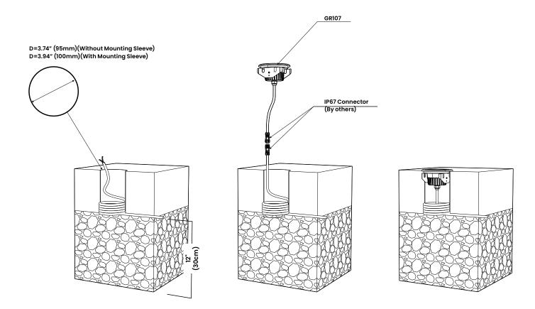
Prepare the ground, providing proper support for the mounting sleeve and install an adequate drainage system according to the application. Pipes may be installed in soft or hard ground to provide adequate drainage. For soft ground installations, drainage material such as pea gravel must be installed to a minimum depth of 12" (30cm). Minimum drainage rate 0.2Gal/min (0.75L/min) Luminaire should be installed only once adequate drainage is confirmed and mounting sleeve is dry and clean of debris.
