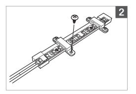
2. Mount clips to surface with screws.
