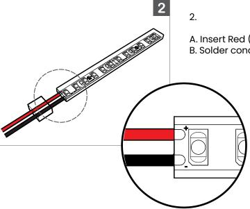
A. Insert Red (+) and Black (-) conductors through End Cap. B. Solder conductors directly onto PCB at assigned location.
