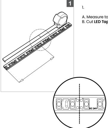
A. Measure to required length of **LED Tape**. B. Cut **LED Tape**.
