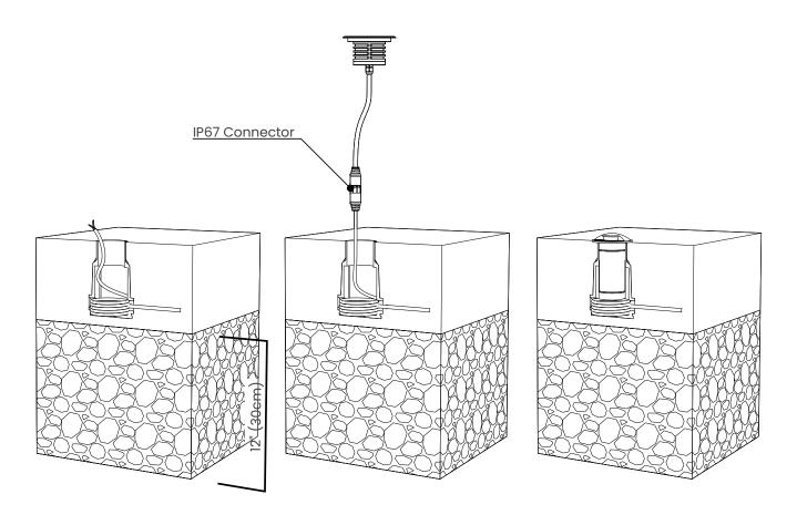
Prepare the ground, providing proper support for the mounting boot and install an adequate drainage system according to the application. Pipes may be installed in soft or hard ground to provide adequate drainage. For soft ground installations, drainage material such as pea gravel must be installed to a minimum depth of 12" (30cm). Minimum drainage rate 0.2Gal/min (0.75L/min) Luminaire should be installed only once adequate drainage is confirmed and mounting boot is dry and clean of debris.
