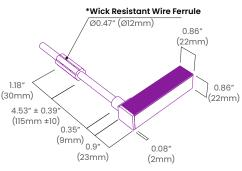
\*The Wick Resistant Wire Ferrule is built into the lead wire, 4.5" (115mm) from the BL Neonview Termination Connection, for additional moisture ingress protection. Removal of the Wick Resistant Wire Ferrule may void your warranty.
