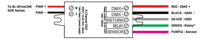
\* The relay must be protected against inductive over voltage spikes, i.e. it must have a flyback diode. Do not connect a typical PCB relay without the diode. RELAY and SENSOR outputs are optional.
