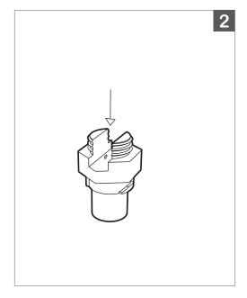
2. Using a small brush, apply Ox-Gard anti-oxidant compound at the bottom of the Lamp Holder where the pins are located.
