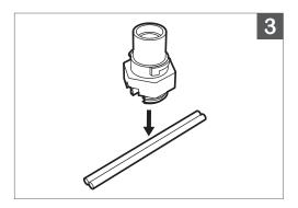
3. Secure Lamp Holder onto the Wire
