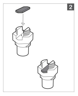
2. Insert the rubber plate into the Lamp Holder
