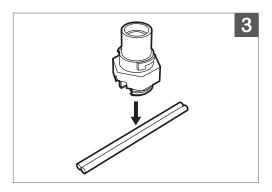
3. Secure Lamp Holder onto the Wire
