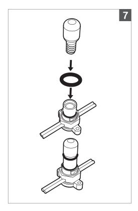
7. Slip the upper(thick) O-ring over the Lamp and Screw the Lamp into the Lamp Holder
