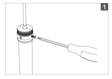
Route Lead Wire through Socket, and fully insert until it touches the end. Secure the Socket to **N360** using (4) screws provided, and tighten until they are flush with the surface of the Socket.
