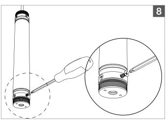
Slip the second O-ring over the end of the N360 light opposite the Lead Wire, and then secure the Socket to the other end of the N360 light, as in Step 1.
