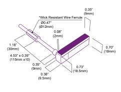
\*The Wick Resistant Wire Ferrule is built into the lead wire, 4.5" (115mm) from the BL neonVIEW Termination Connection, for additional moisture ingress protection. Removal of the Wick Resistant Wire Ferrule may void your warranty.
