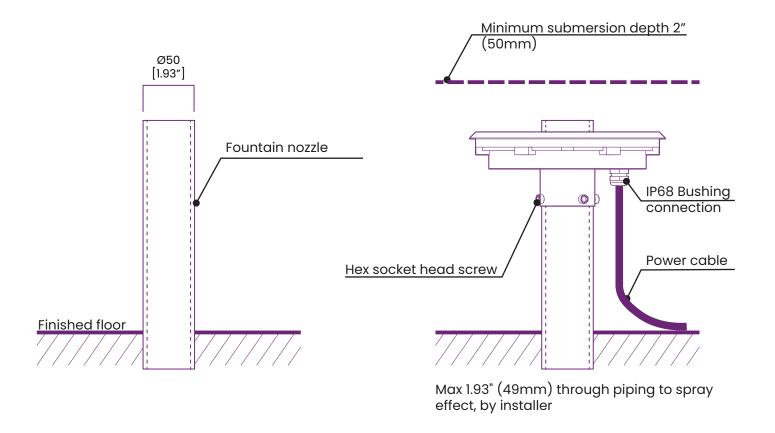
IMPORTANT: The joint of wiring connection between fixture and main power must be IP68 waterproofed.
