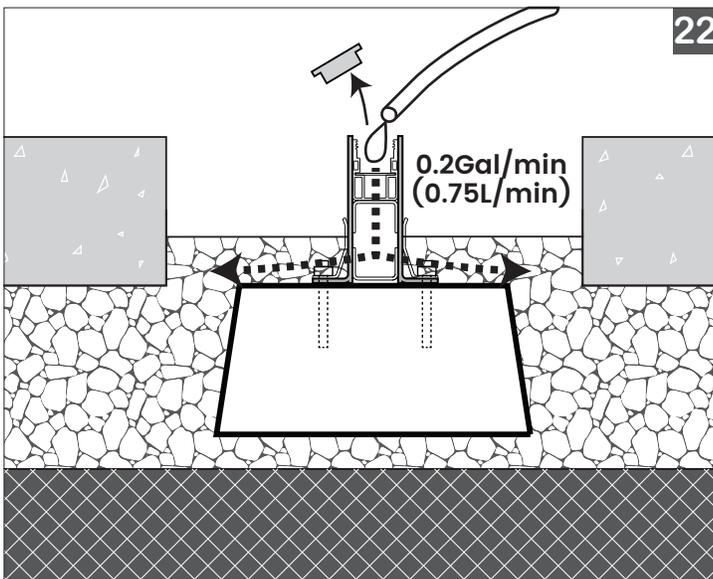
22. Remove the Knockout Cover and test for adequate drainage using a hose or a bucket of water. Minimum drainage rate 0.2Gal/min (0.75L/min). Luminaire is not meant for permanent submersion in water and should be installed only once adequate drainage is confirmed.
