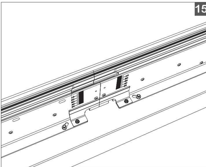
15. Fastening points are located on the flanged Channel base.
