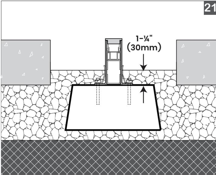
21. Ensure the bottom sides of the Channel are always situated in a permeable layer, of 1-1/4" (30mm) from top of concrete footing to the top of the permeable fill layer to ensure good drainage.
