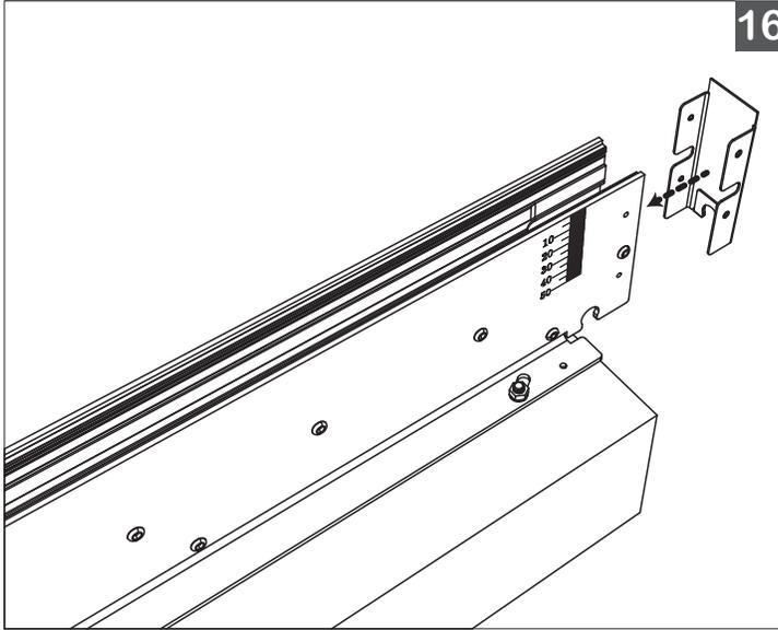
**16.** Secure End Cap to the last Channel in line.
