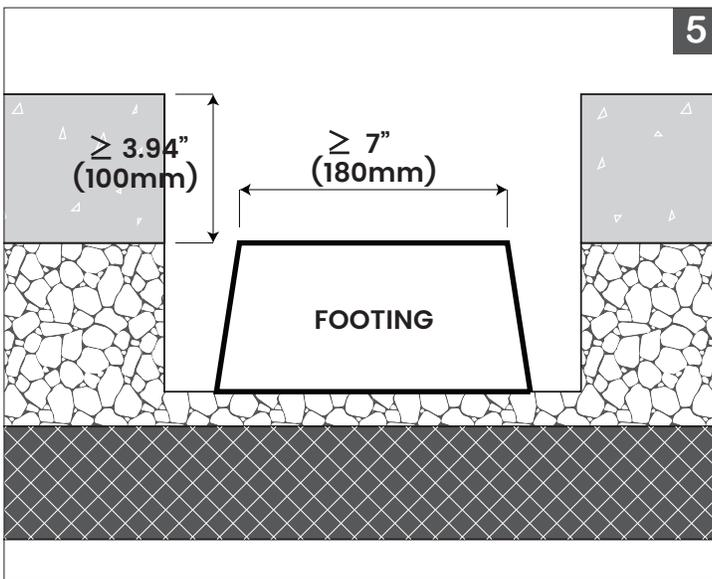
**5.** The concrete footing must be level and of adequate size to support the luminaire along the entire length, and to fix the luminaire directly to the footing with expansion bolts.
