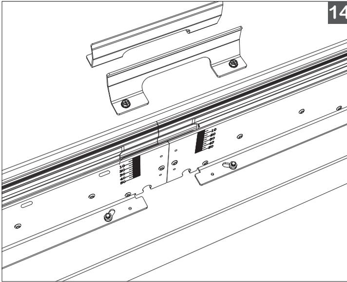
14. Secure Channel in place, and maintain secure connection and alignment with subsequent channel lengths using the Channel Connector Brackets.
