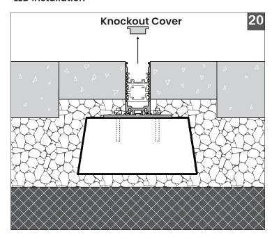
20 & 21. Carefully remove the Knockout Cover.
