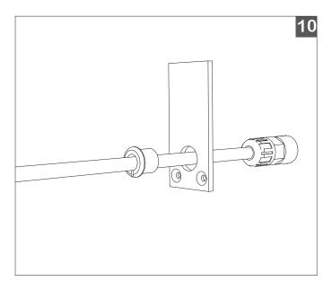
10 & 11. Slip the Bushing over the wires, slide to the End Cap and seat in place.
