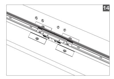
14. Ensure fasteners are secure, and not over-tightened.
