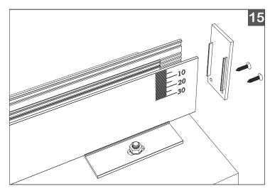
15. Secure End Cap to the last Channel in line.
