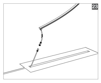
Carefully lay the LED into the Channel, starting from the power input end.
