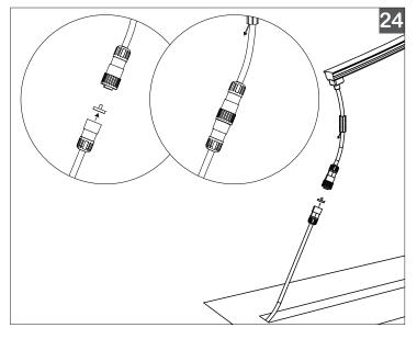
24. Verify wiring to the LED Driver, remove protective end cap, and connect to power using Quick Connects and test.
