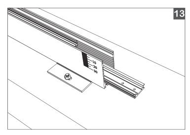
12 &13. Secure Channel in place, and maintain secure connection and alignment with subsequent channel lengths using the Channel Connector Brackets.
