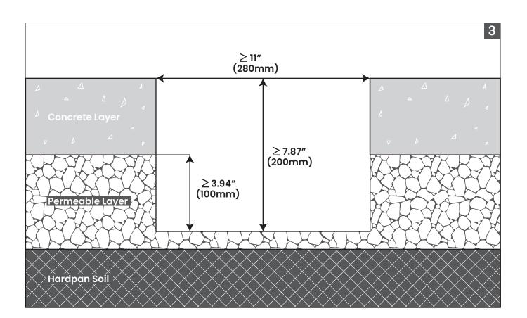
3. Depth of cutout in ground surface will depend upon the depth of permeable layer, concrete top layer, and concrete footing size required.
