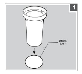
1. Create hole for recessing **DISK114** with a 4" OD. The recessed depth must align **DISK114** flange flush to ground level.
