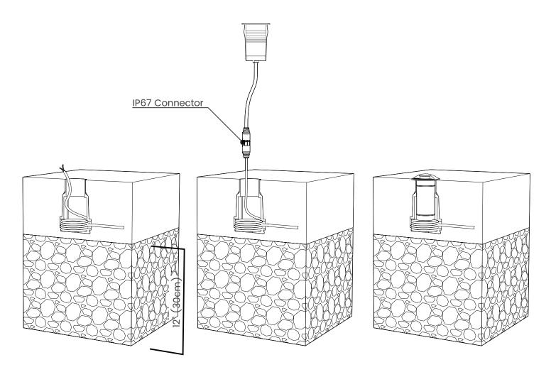
Prepare the ground, providing proper support for the mounting boot and install an adequate drainage system according to the application. Pipes may be installed in soft or hard ground to provide adequate drainage. For soft ground installations, drainage material such as pea gravel must be installed to a minimum depth of 12" (30cm). Minimum drainage rate 0.2Gal/min (0.75L/min) Luminaire should be installed only once adequate drainage is confirmed and mounting boot is dry and clean of debris.
