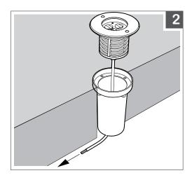
2. Install boot and run wiring.
