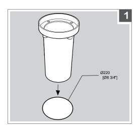
1. Create hole for recessing **DISK \$250** with a 8 3/4" OD. The recessed depth must align **DISK \$250** flange flush to ground level.
