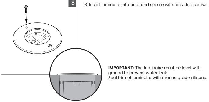
**IMPORTANT:** The luminaire must be level with ground to prevent water leak. Seal trim of luminaire with marine grade silicone.
