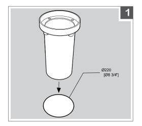
1. Create hole for recessing **DISK R250** with a 83/4° OD. The recessed depth must align DISK R250 flange flush to ground level.
