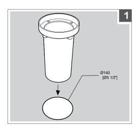
1. Create hole for recessing **DISK R150** with a 5 1/2° OD. The recessed depth must align DISK R150 flange flush to ground level.
