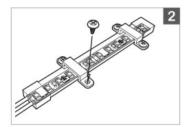
2. Mount clips to surface with screws.
