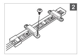
2. Mount clips to surface with screws.
