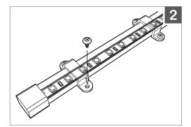
2. Mount clips to surface with screws.
