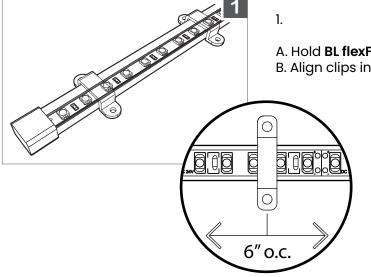
A. Hold **BL flexFORM LINE DI Series** taught to mounting surface.B. Align clips in-between LED diodes (not directly over them).
