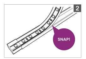
2. Push **BL flexFORM LINE DI Series** into PVC Track for snug and secure fit.
