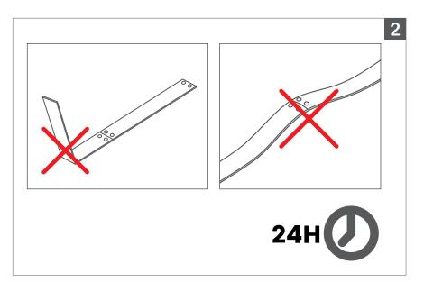
2. Secure BL flexFORM LED TAPE gently along the length, without bending or pulling up.
