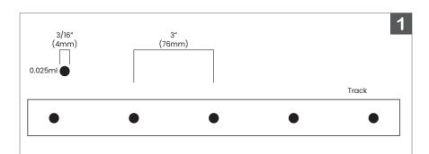
1. Place a small dab (0.025ml) of adhesive onto the inside ridge of the BL fixFORM base track channel at 3" intervals.
