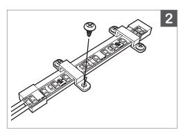
2. Mount clips to surface with screws.
