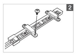
2. Mount clips to surface with screws.
