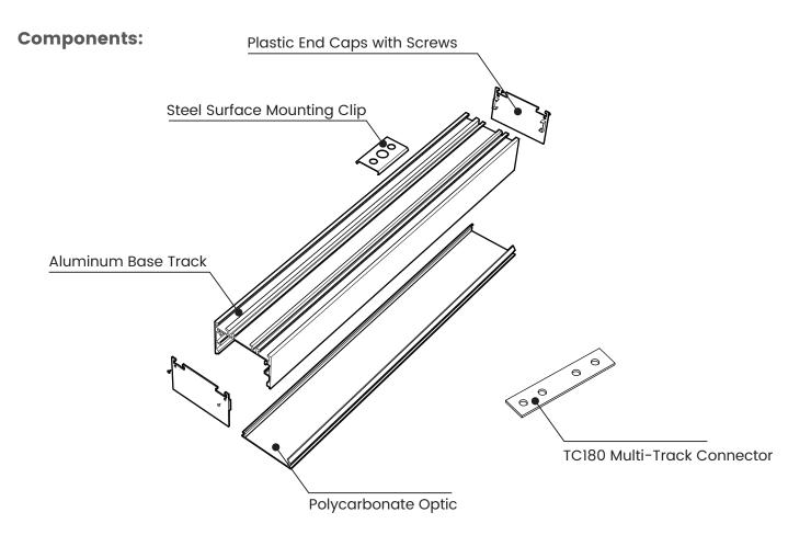
BL fixFORM SF WIDE is designed to house two side by side lengths of BL flexFORM LED Tape.
