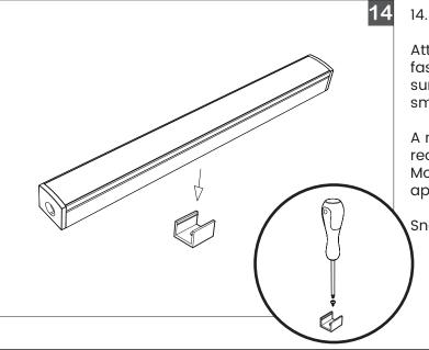
Attach the included Mounting Clips using fasteners appropriate for your mounting surface, which should be clean, dry and smooth.
