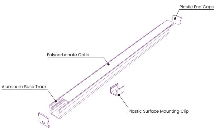
Each 8ft length of LED Profile is shipped complete with End Caps, and Mounting Clips.
