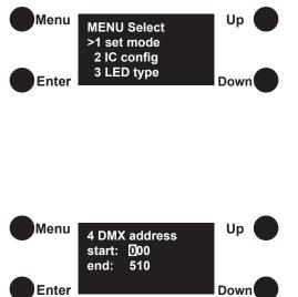
Press the "Menu" button to access the menu selection interface. Use the "Up" and "Down" buttons to select the specific settings. Use the "Enter" button to access the setting sub-menu. Use the "Up" and "Down" buttons to change the settings and press "Enter" to select the desired option or to move to the next figure when changing number values, such as DMX address. Press the "Menu" button to confirm the setting and return to the selection screen.
